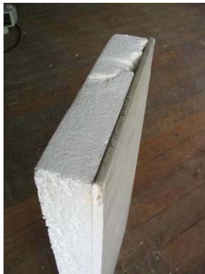
Figure 11. Wall insulation system: Expanded Polystyrene with Gib.
