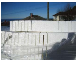
Figure 16. New underfloor insulation: Expanded polystyrene sheets.
