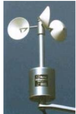
Figure 6. Site Wind Speed Measurement Device
