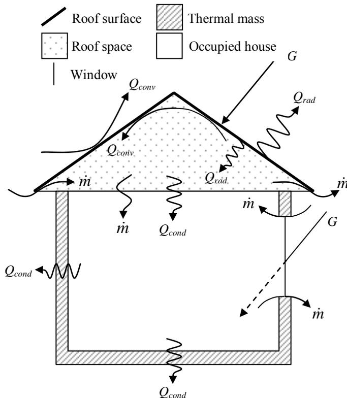
Figure 1. Schematic diagram of the modelled system with energy transfer components shown.
