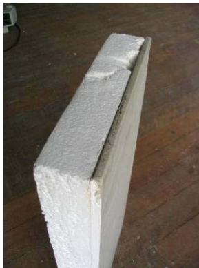
Figure 11. Wall insulation system: Expanded Polystyrene with Gib.
