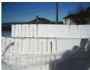
Figure 16. New underfloor insulation: Expanded polystyrene sheets.
