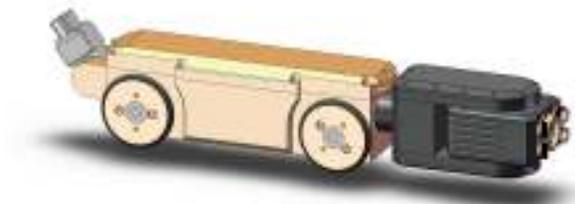
**Figure 12a:** Fully assembled robot with military grade connection plug at rear
