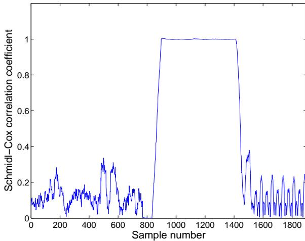
Figure 5: Schmidl-Cox detection algorithm increases from 0 to 1 as the packet is received at sample number 900
