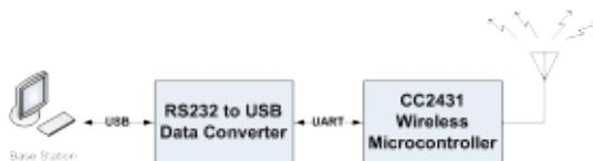
Figure 6: Base station with coordinator node
