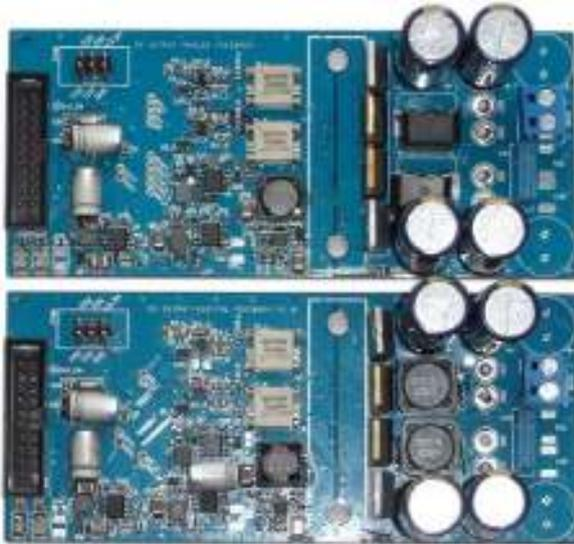
Figure 7: Prototype Analogue (Top) and Digital (Bottom) One-Cycle Control Boards - Top View
