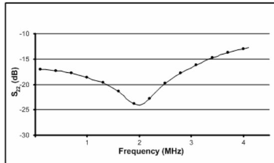
Fig. 10. Output reflection coefficient  $S_{22}$ .
