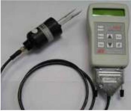
Figure 4: Delta-T HH2 Commercial Soil Moisture Sensor
