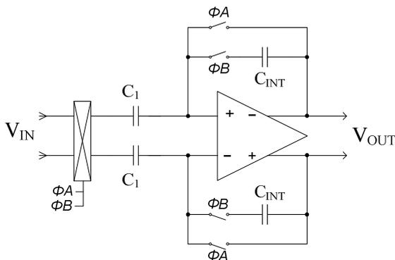
Fig. 4. Switched-capacitor integrator using correlated double-sampling.
