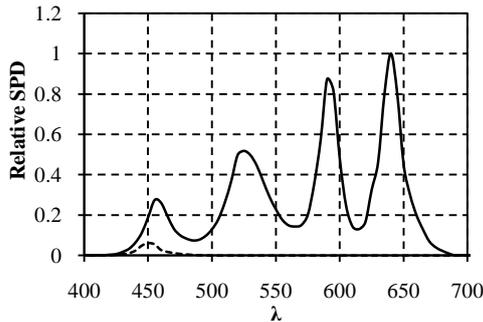
Figure 10: SPD of the optimised mixture of the royal-blue  $\lambda_{rb} = 450$  nm, blue  $\lambda_b = 460$  nm, green  $\lambda_g = 530$  nm, amber  $\lambda_a = 590$  nm and red  $\lambda_r = 630$  nm LEDs:  $R_a = 96$ ,  $R_b = 86$ ,  $\eta_{rad} = 338$  lm/W, CCT = 3356K,  $R_{12} = 75$  (the blue test sample).
