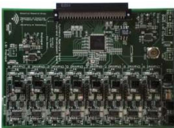
Figure 5: The PCB designed to evaluate the front-end. The AD9271 is the IC next to the connector.
