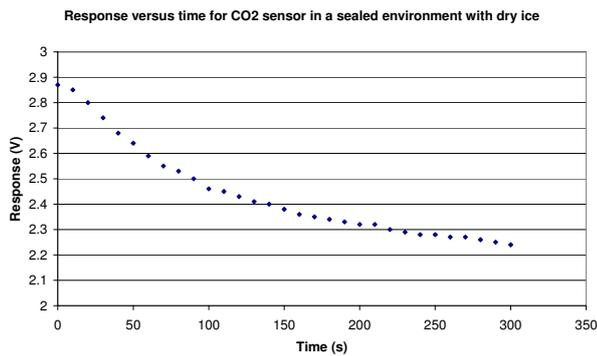
Figure 10: CO<sub>2</sub> sensor response to sublimating dry ice
