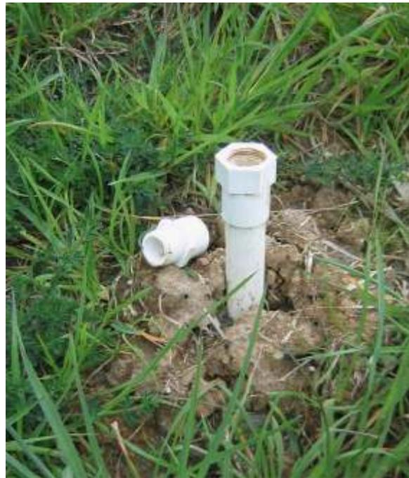
Figure 4: All that can be seen from the surface of one stand pipe
