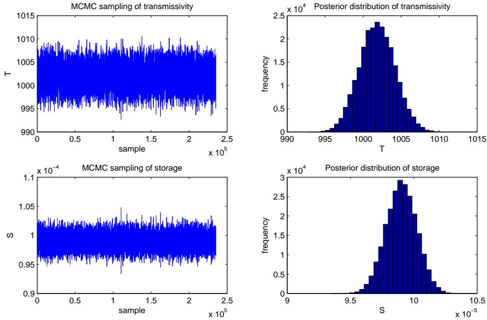
Figure 5: T-walk sampling for the Theis model, after burn-in. Left: output traces of transmissivity  $T$  (top) and storage  $S$  (bottom). Right: posterior histograms for transmissivity  $T$  (top) and storage  $S$  (bottom).
