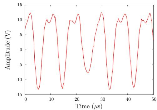
Figure 6: The output of the class D amplifier for a 110 kHz sinusoid with a supply voltage of 30 V.
