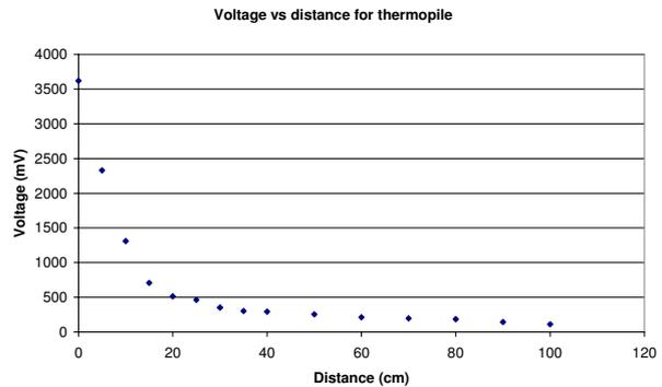
Figure 3: Characteristic response of ZTP-135S thermopile
