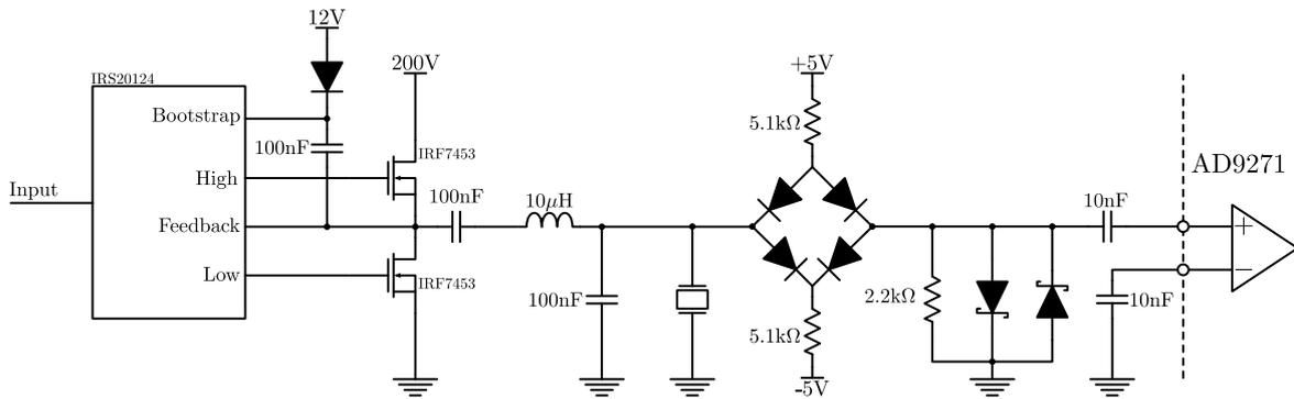
Figure 4: The front-end for a single channel. The transmitter is shown to the left of the transducer while the T/R switch on the right leads into the inputs of the AD9271.
