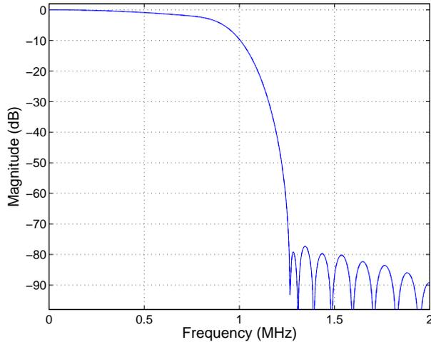
Figure 3: Combined receiver CIC-HBF filter response from DC–2MHz, with a decimation rate of 32. [3]
