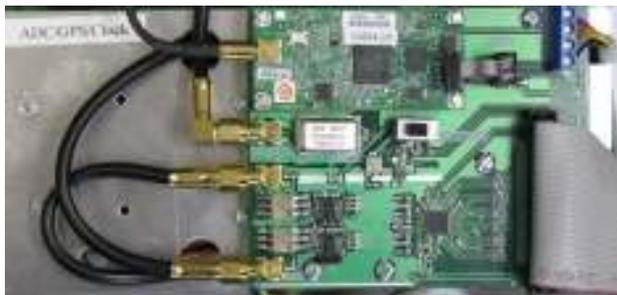
**Figure 7:** ADC, GPS and Precision Clock module
