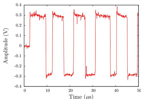
Figure 7: The output of the T/R switch when the transmitter is outputting a 110 kHz, 30 V<sub>p-p</sub> sinusoid.
