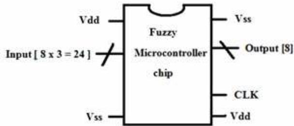
Figure 8: Input/Output pin definition for the fuzzy microcontroller chip
