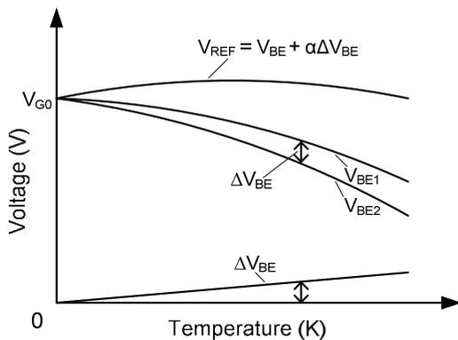
Fig. 1. The temperature characteristics of the base-emitter junction voltage  $V_{BE}$ , and the derived voltages  $\Delta V_{BE}$  and  $V_{REF}$ .
