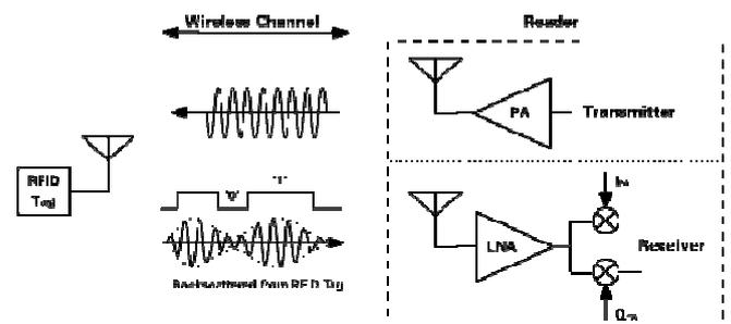
Fig.1 The Simulation Environment of Return Link for RFID system (Receiver, Wireless channel, and Tag)
