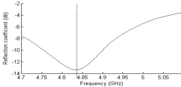
Figure 9. Reflection coefficient. Middle frequency is shown by vertical line is 4.84GHz
