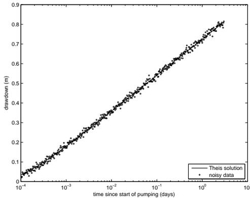
Figure 4: Synthetic pump test data for the Theis model
