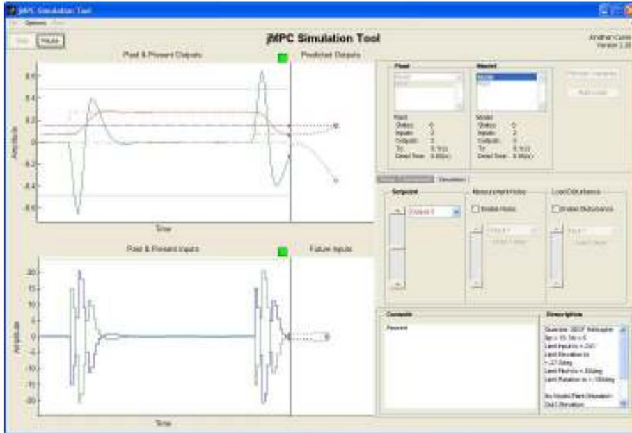
Figure 5: The Model Predictive Control graphical user interface controlling a 3 DOF Quanser helicopter. Note the depiction of the future input and output predictions.
