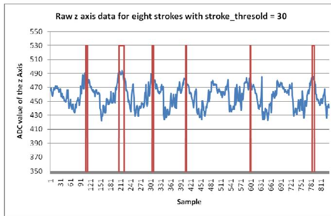
Figure 5 - 8 real-world kayak strokes with overlaid stroke detection
