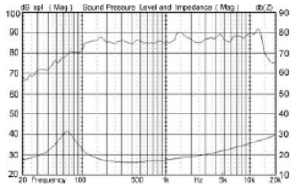
Figure 7: Frequency response of W4-654S speaker [8]
