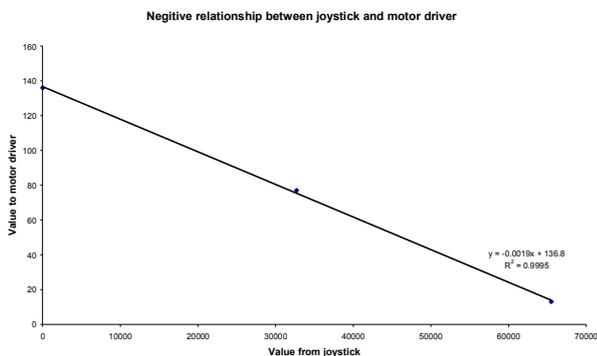
**Figure 8:** Relationship for forward direction of joystick, relating to driving of robot, output versus input.
