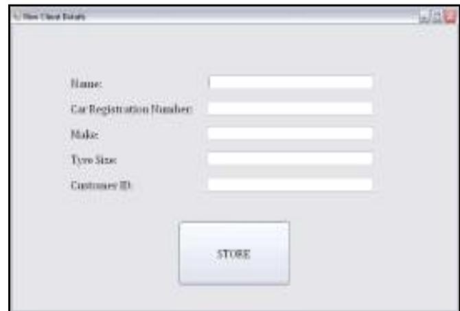
The above is a snapshot of the Client Details Storage Window. Here the basic details like the Name, Registration Number of the vehicle, its make, the tyre size and the Customer ID is stored. When the 'Store' button is clicked, the details are stored into a table called 'client' in the database.
