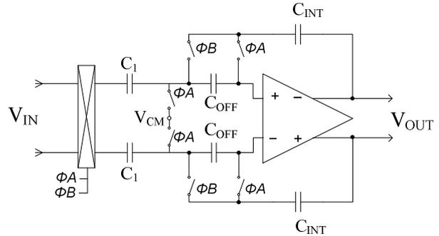
Fig. 6. Improved CDS integrator with minimal charge leakage.
