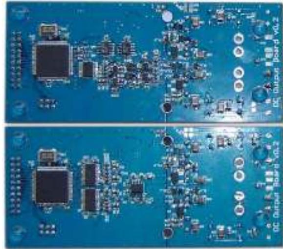
Figure 8: Prototype Analogue (Top) and Digital (Bottom) One Cycle Control Boards - Bottom View
