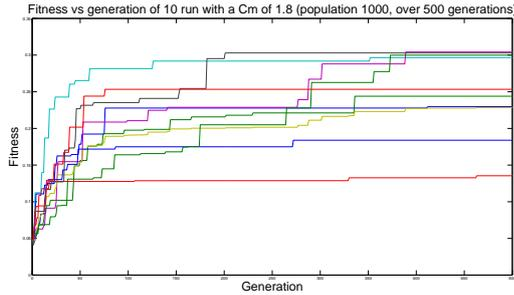
Figure 1: Typical results from 10 GA runs using linear scaling.
