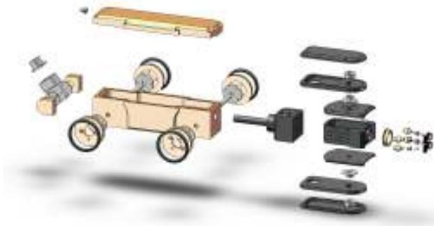
**Figure 12b:** Exploded view of the same robot, displaying the full extent of seals that need to be replaced and the overall complexity of the unit.
