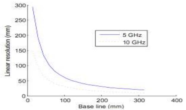
Figure 12. Dependencies of linear resolution for two frequencies 5 and 10 GHz from the distance between antenna elements
