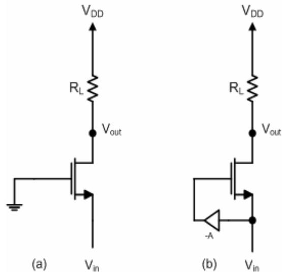
Fig.1. (a) Conventional CG amplifier, and, (b)  $g_m$ -boosted CG amplifier.
