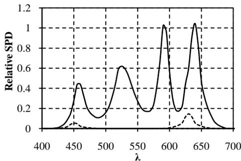
Figure 11: The 6-band light source with the royal-blue  $\lambda_{rb} = 450$  nm, blue  $\lambda_b = 460$  nm, green  $\lambda_g = 530$  nm, amber  $\lambda_a = 590$  nm, red-orange  $\lambda_{ro} = 630$  nm and red  $\lambda_r = 630$  nm LEDs:  $R_a = 96$ ,  $R_b = 86$ ,  $\eta_{rad} = 338$  lm/W, CCT = 3356K,  $R_{12} = 75$  (the blue test sample).
