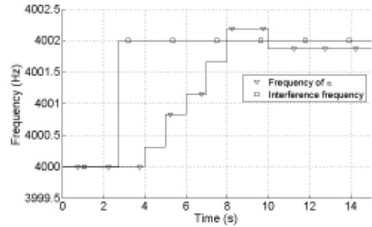
Figure 10: Step response of the tracker in simulation.
