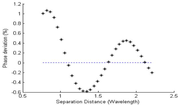
Figure 13. Dependency for possible error value in the phase measurements due to mutual coupling from the distance between two antenna elements.
