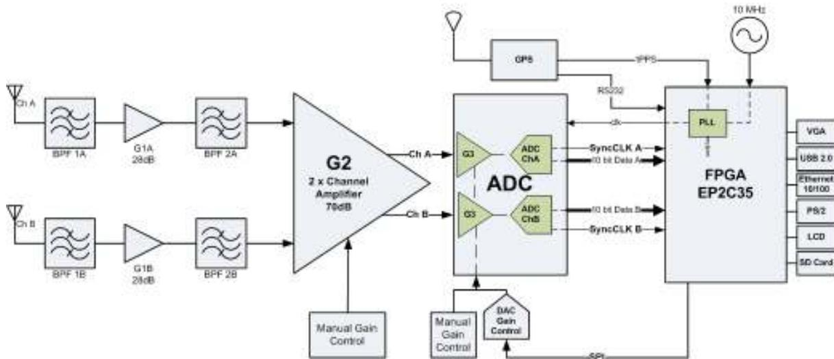
Figure 5. DRS functional block-diagram
