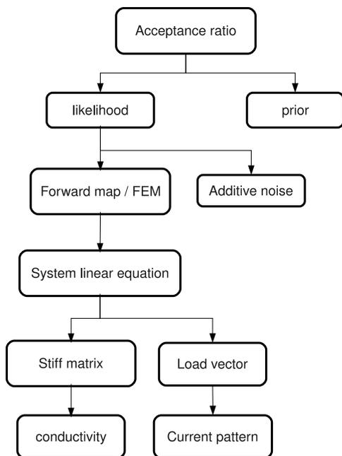
Figure 5: Diagram of computational steps for the acceptance ratio
