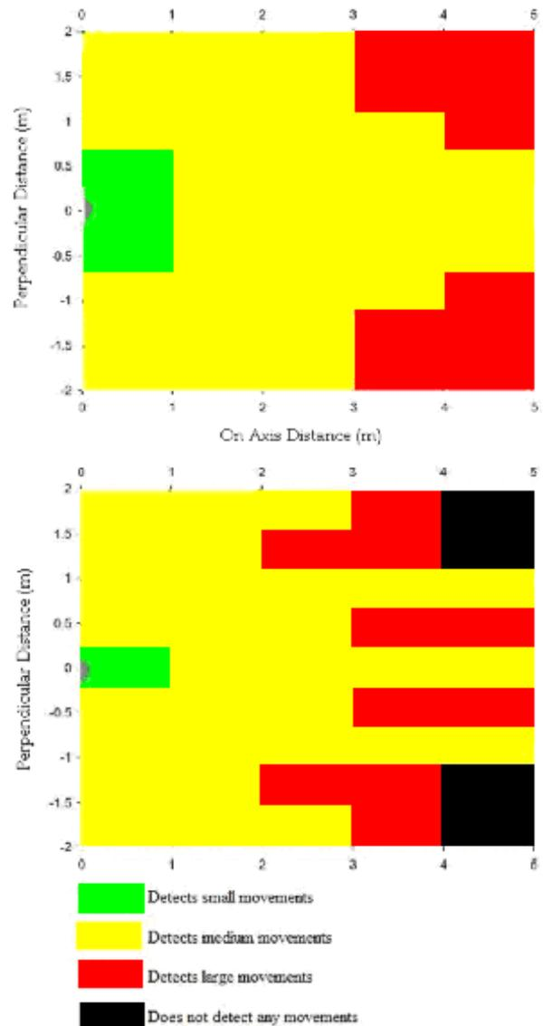
Figure 14: Motion detector response in dark (top) and bright (bottom) conditions
