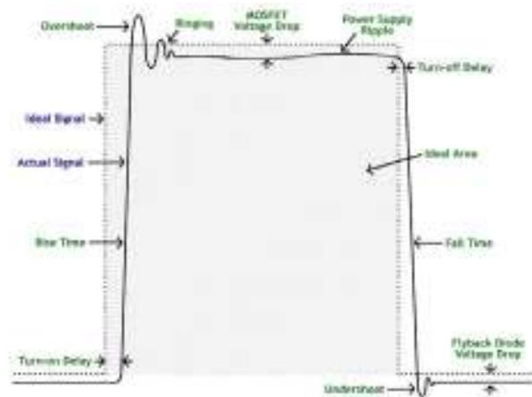
Figure 3: Sources of Error in the Switching Converter
