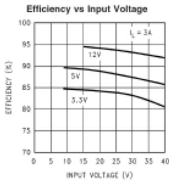
Figure 4: Efficiency of LM2676T at maximum current through-put for different input and output voltages.
