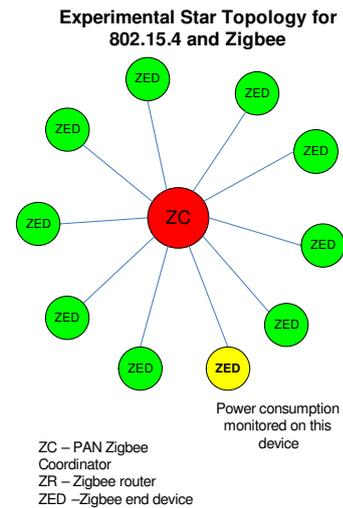
Figure 3: IEEE 802.15.4 and Zigbee star network topology
