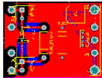
Figure 2b: PCB layout of power module protection board showing slot-in design and isolation of 300 VDC input
