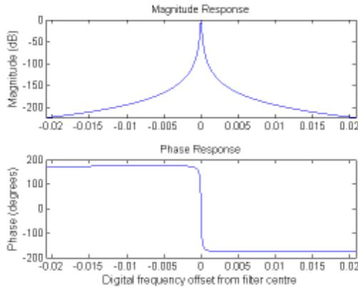
Figure 5: Frequency response of second order filter.
