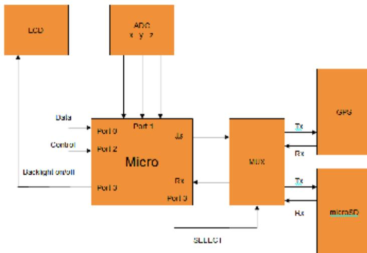
Figure 2 - Operational diagram of the WaterLogged device
