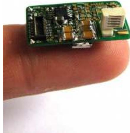
Figure 1: Bird-tag that uses the GPS FastFix algorithm to improve battery life and reduce size and mass.
