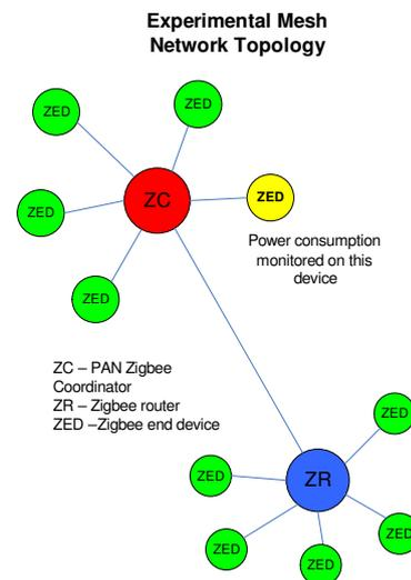
Figure 4: Zigbee mesh network topology
