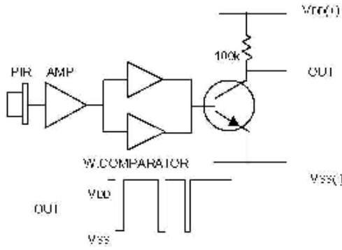
Figure 4: MS401 motion detector internal circuit
