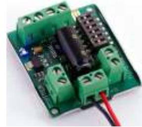
Figure 5: Sabertooth 2×5 Motor Driver unit<sup>[7]</sup>
