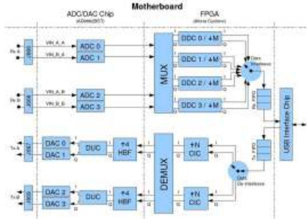
Figure 2: ADC/DAC and FPGA sections of the USRP, showing the sampling conversion stages and the multiplexer used for routing data. [1]
