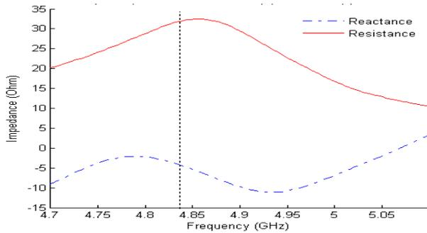
Figure 8. Result acquired with network analyser. The Impedance Resistance and Reactance components. Middle frequency shown by the vertical line is 4.84GHz
