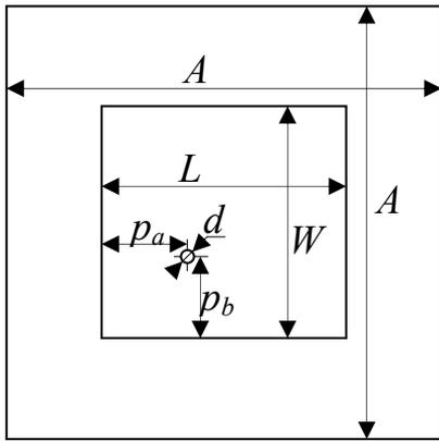
Figure 1. Near square patch antenna sketch and variable dimensions for selected basic antenna design
