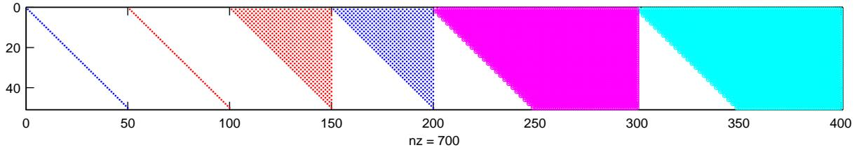
Figure 1: The sparsity pattern and structure of the constraint matrix,  $\mathbf{A}^T$  in the MPC formulation given in Eqn. 2. The blue symbols are positive values; red negative.
