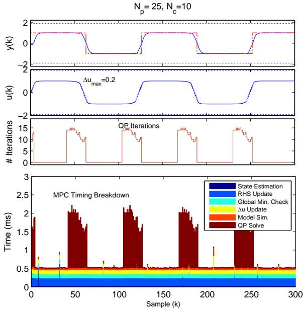
Figure 4: Timing breakdown of an MPC implementation for a SISO non-minimum phase (inverse response) application.
