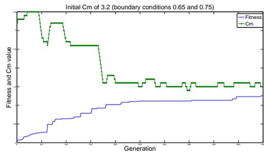
Figure 5: GA with dynamic linear scaling showing how  $C_m$  changes over the generations.
