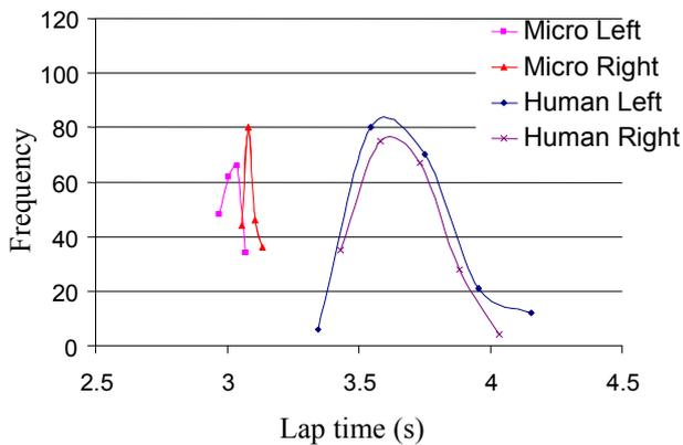
Figure 9: Plot of the frequency of lap times achieved by car and expert on left and right lanes of the test track. The consistency of the slot car compared with a skilled human clearly reveals the difference between the lanes.
