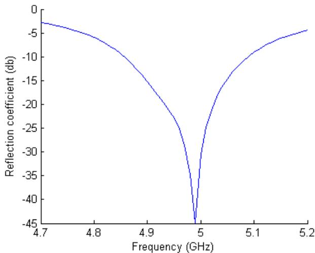
Figure 6. Final results of the mathematical modelling. Reflection coefficient is below -20db
