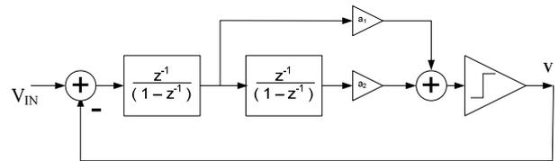
Fig. 3. Second-order CIFF loop structure used as the  $\Delta\Sigma$  modulator.
