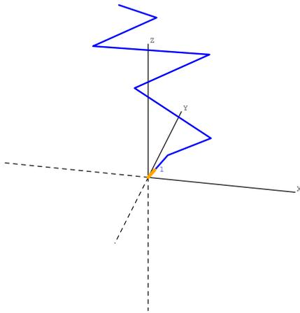
Figure 8: Best individual after 1000 generations with dynamic linear scaling. The GA has ‘discovered’ a helix-like structure for the reception or RHCP signals.
