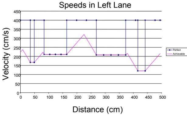
Figure 2 Plot of ideal (joined dots) and achievable (light continuous lines) velocity of a car as a function of distance around the left lane of the track shown in figure 1.
