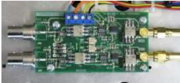
**Figure 6:** Two Channel Amplifier G2 module
