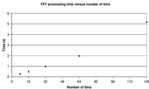
Figure 13: FFT processing time versus bin size using the AT89C51AC3 microcontroller
