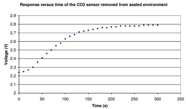
Figure 11: CO<sub>2</sub> recovery characteristic
