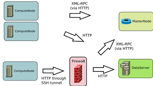
Figure 5: OGRE’s SSH-tunneling scheme to pass through restrictive firewalls.
