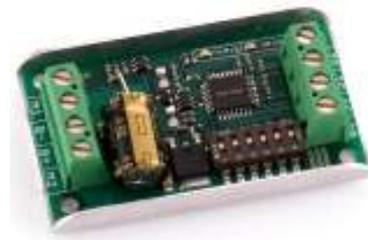
Figure 6: SyRen10 Motor Driver unit<sup>[7]</sup>
