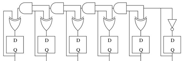
Figure 2: Radix-2 counter with carry chain (clock and reset signals omitted)
