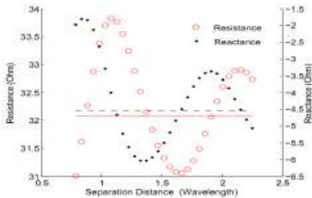
Figure 11. Coupling. Dependence of the Real and Imaginary parts of the mutual impedance from the distance between two antenna elements. Horizontal dashed line represents value for the Imaginary part for the single antenna and solid line correspondent value for the Real part.
