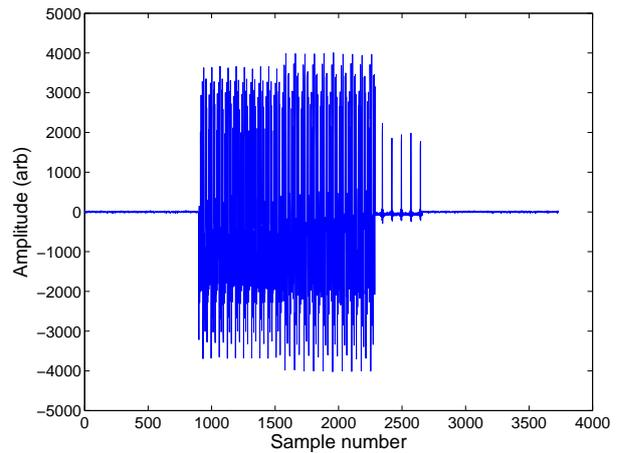
Figure 6: CFO derotated received waveform starting at sample number 900, showing the three distinct sections of the sounding sequence.
