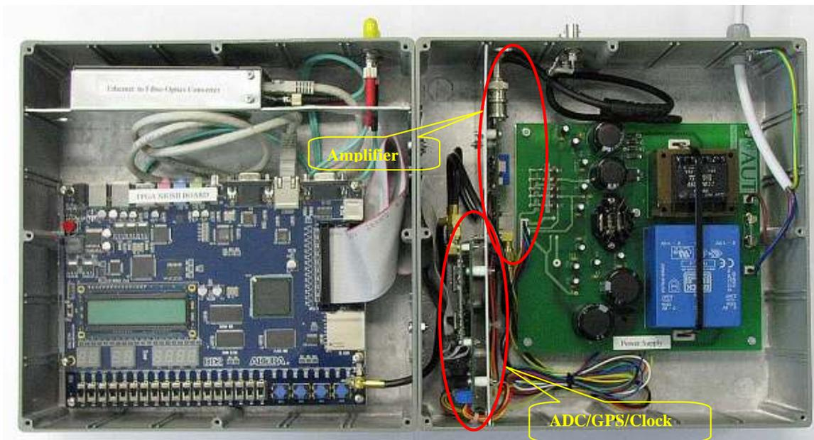
Figure 6. Assembled DRS. The box on the left contains digital elements of the system with 100MHz fibre-optical data transmission line to reduce harmful interferences to the antenna and analogue electronics.
