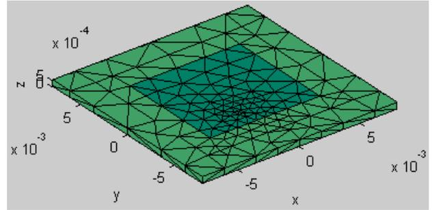
Figure 3. 3-D model of patch antenna. All dimensions are shown in m.
