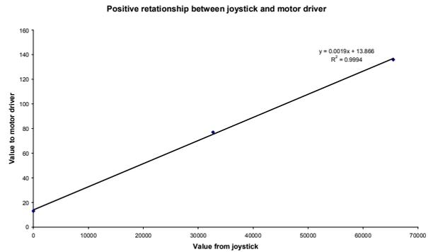
**Figure 9:** Relationship for twist and sideways directions of joystick, relating to control of camera motors of robot, output versus input.
