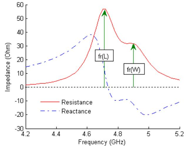
Figure 4. Modelled parameters for initial dimensions given in the Table 1. Two resonance picks pointed by arrows  $fr(L)$  and  $fr(W)$  related to effective dimensions of our patch  $L_e$  and  $W_e$  correspondently.
