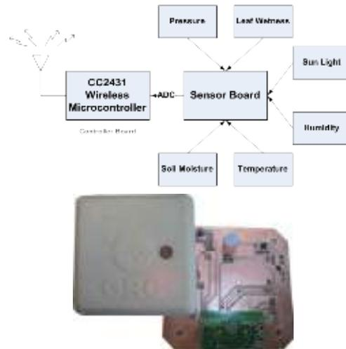
Figure 7: Router node with environmental sensors
