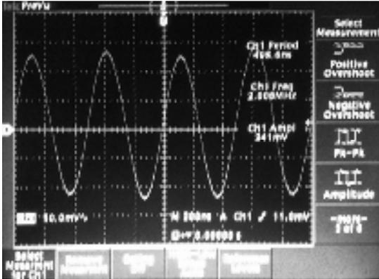
Fig. 5. Oscilloscope trace of 2 MHz tone test at the output of the amplifier.
