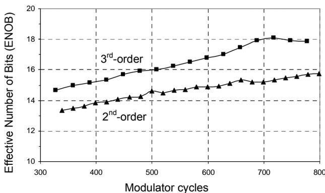
Fig. 7. Plot of output resolution vs. total modulator cycles for symmetric second-order and third-order decimation filters.
