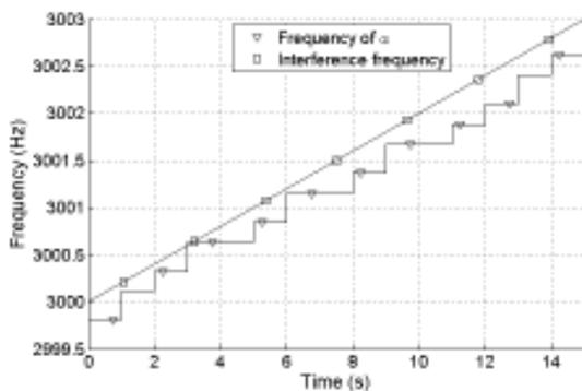
Figure 9: Operation of tracker with interference tone and noise.
