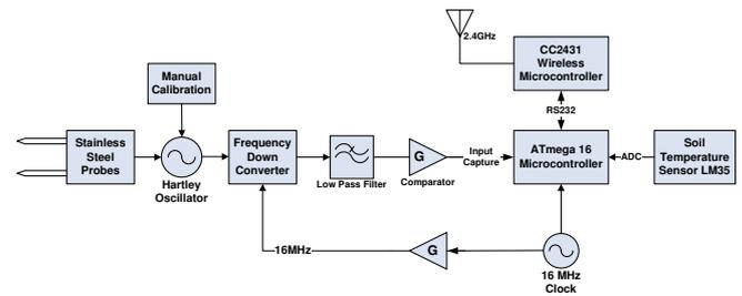
Figure 3: Soil Moisture Sensor Block Diagram
