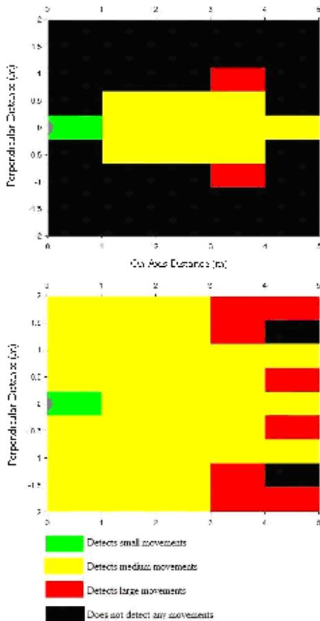
Figure 5: Characteristic response of MS401 motion detector with (top) and without (bottom) paper sheave
