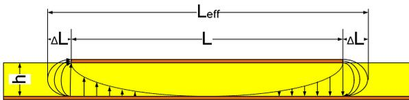
Figure 2. Effective patch dimensions are greater than its physical dimensions
