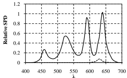
Figure 9: SPD of the optimised mixture of the blue  $\lambda_b = 460$  nm, green  $\lambda_g = 530$  nm, amber  $\lambda_a = 590$  nm, red-orange  $\lambda_{\text{ro}} = 630$  nm and red  $\lambda_r = 630$  nm LEDs:  $R_a = 95$ ,  $R_b = 85$ ,  $\eta_{\text{rad}} = 343$  lm/W, CCT = 3269K,  $R_9 = 75$  (the red test sample).
