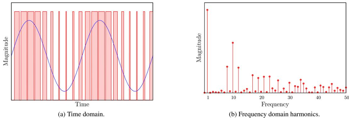
Figure 3: The class D waveform for a sinusoidal signal.
