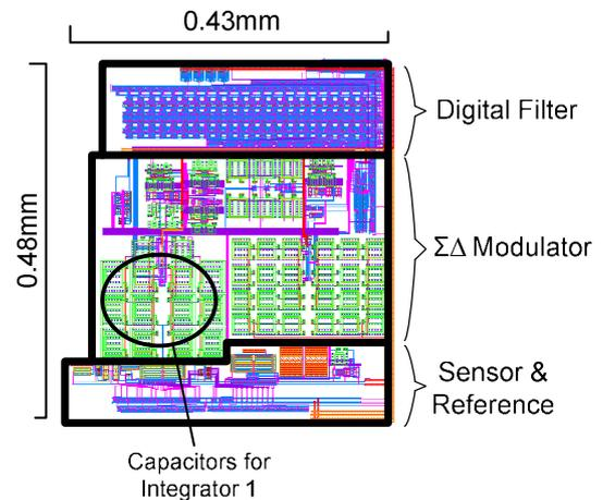
Fig. 8. Layout of the complete smart temperature sensor.
