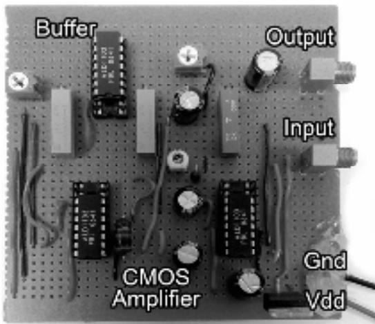
Fig.4. Amplifier test board with output buffer and SMA input output connectors.
