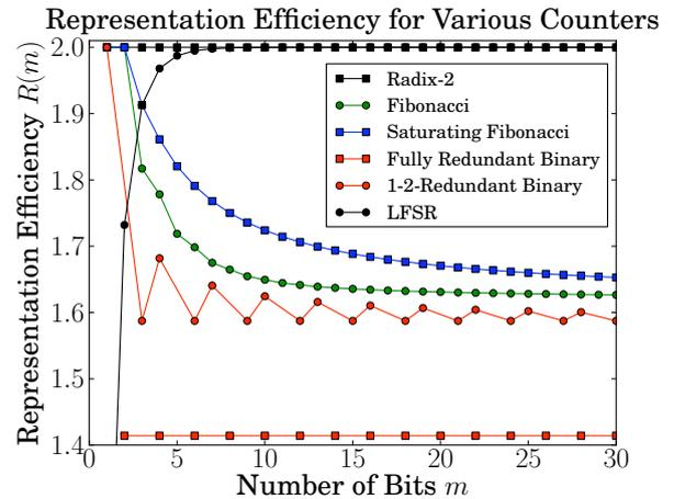
Figure 5: Representation efficiency for counter sizes up to 30 for the radix-2 counter (Section 3), Fibonacci counter (Section 2), Saturating Fibonacci Counter (Section 7.1) and the counters in Section 6
