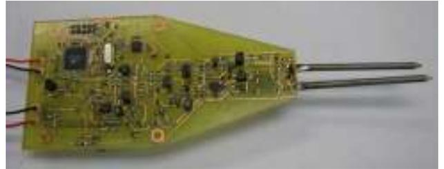
Figure 6: Soil Moisture Sensor
