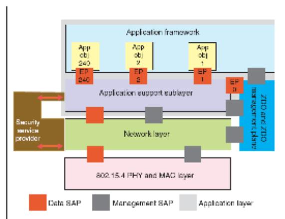
Figure 1: ZigBee stack layer adapted from [5]
