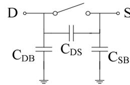
Fig. 5. Parasitic capacitances of a MOS switch.
