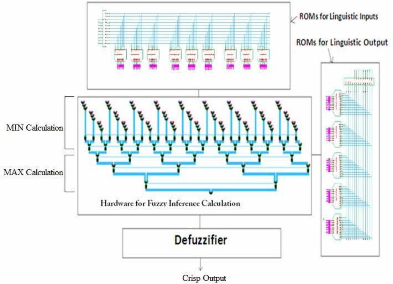
Figure 6: Schematic of hardware architecture of Fuzzy Wash time controller for Washing machine
