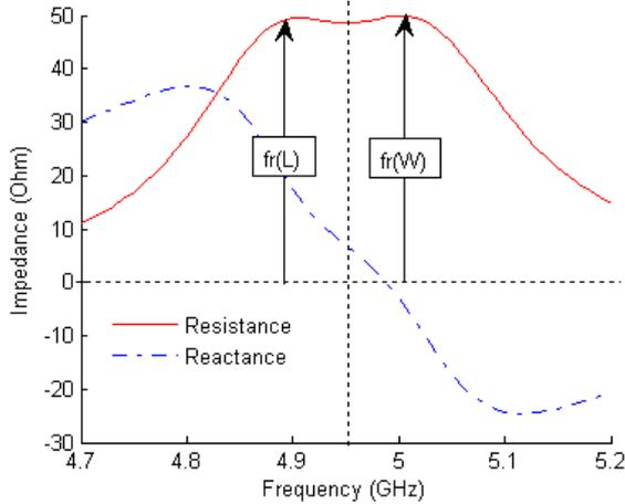
Figure 5. Final results of the mathematical modelling. Active impedance  $R_{in}=50\Omega$  equal for both resonance frequencies
