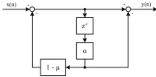
Figure 2: Notch filter structure.
