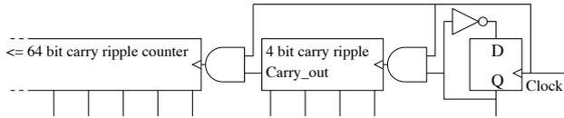
Figure 4: Constant time radix-2 counter. The carry out from each stage is ANDed with the clock signal to form the clock for the next stage
