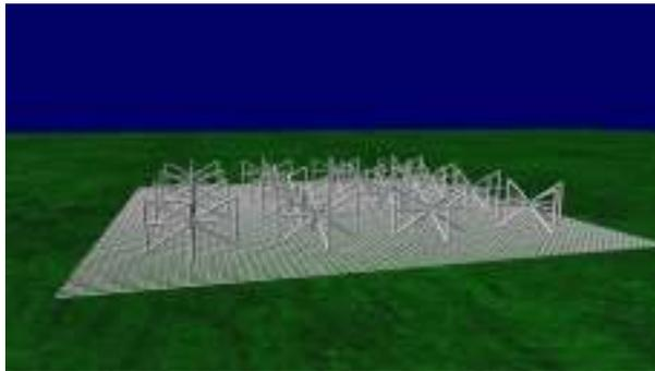
**Figure 2.** Computer model of one of the possible solutions for TREAD-P station. The approximate dimensions of the station on the ground are 10.5x10.5 m.
