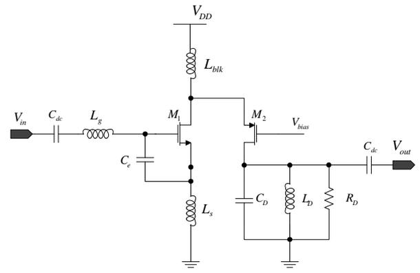
Fig.3 The folded-cascode LNA topology
