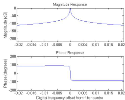
Figure 4: Frequency response of first order filter.
