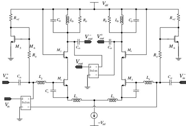
Fig. 4 The differential LNA topology
