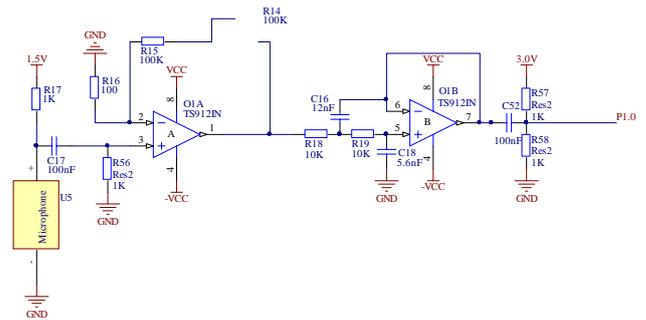
Figure 6: Microphone circuit schematic
