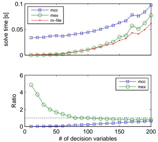
Figure 3: Comparing the timing of an auto-generated C code (`mcc`) implementation of Wright's QP, a hand-coded C implementation (`mex`), and an optimised MATLAB m-file implementation.
