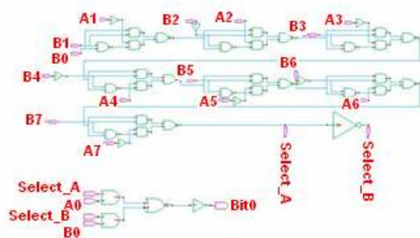
Figure 5: Logic Design of a MIN (MAX) Circuit
