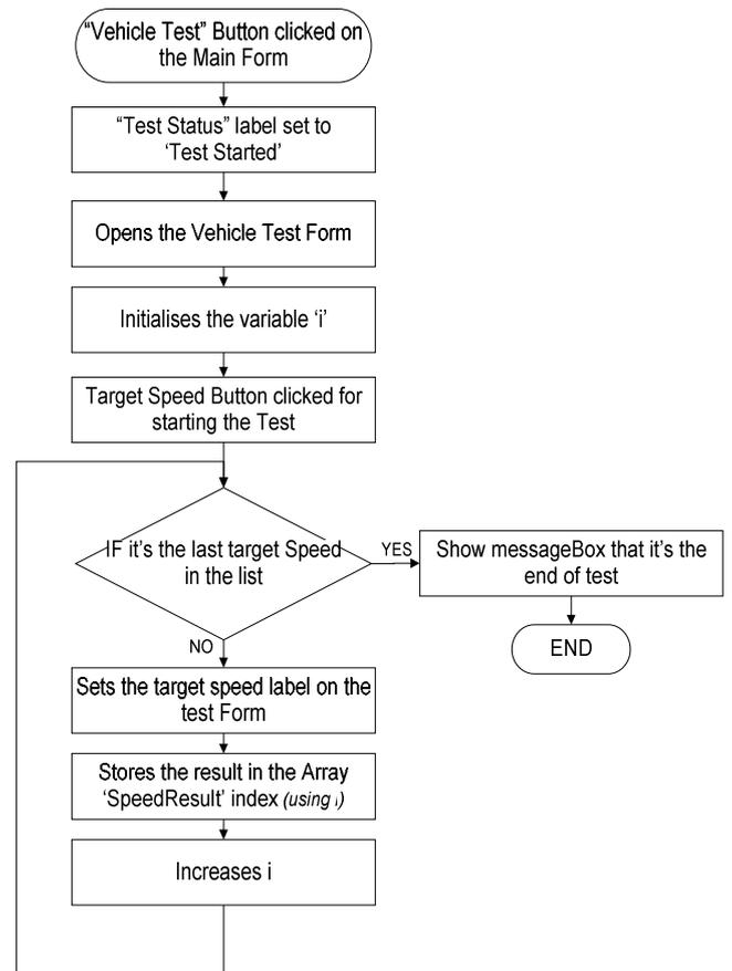
The above is the basic working of the vehicle testing window. There is a 'BACK' button on the testing form that can be used to back to redo the previous speeds of the test.
