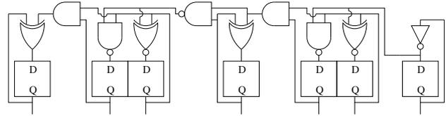
Figure 6: Hybrid redundant binary counter
