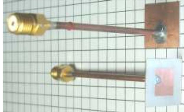
Figure 7. Antennas used in measurements. Dimension of the grid cell is 5x5 mm.
