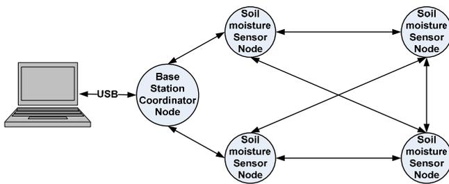
Figure 5: Mesh Network Topology Used in the Soil Moisture Experiment Setup
