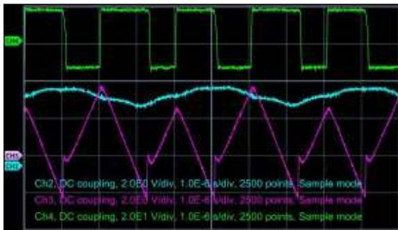
Figure 9: Sub-harmonic Oscillation in Analogue Feedback
