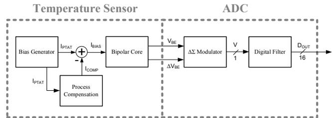
Fig. 2. Block diagram of the smart temperature sensor.
