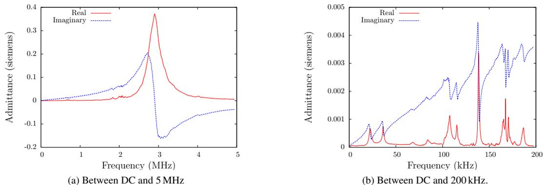
Figure 1: The admittance of the transducers.
