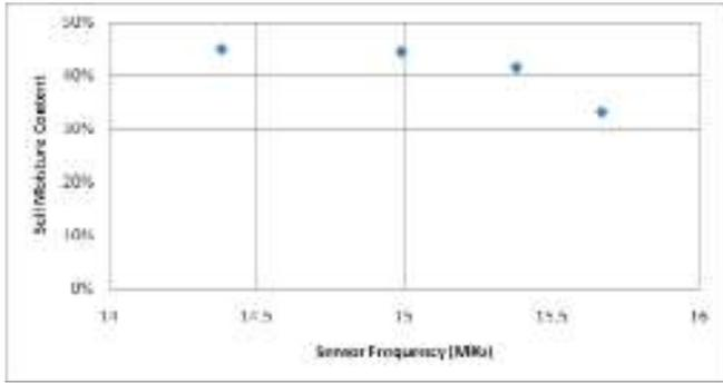
Graph 1: Soil Moisture Content vs Sensor Frequency
