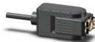
**Figure 11a:** Assembled view of the robots camera head, mid section is connected to a motor so that the camera is able to be panned.
