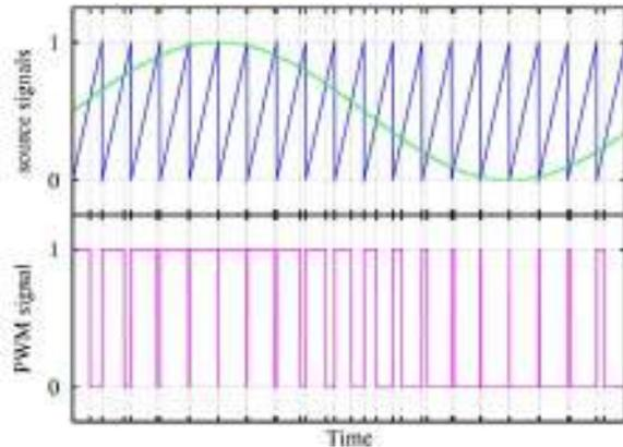
Figure 1: Source, reference triangle wave and resulting PWM signals.
