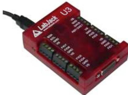
This module acquires signals and waveforms and processes them to obtain desired information for further analysis by a computer by using a vendor supplied software or various programming languages like Java, Visual Basic, C, C++, C# and many others.
