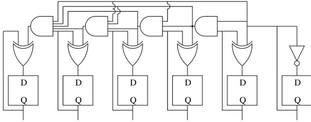
Figure 3: Radix-2 counter with lookahead carry (clock and reset signals omitted). The multiple input AND gates could be replaced by a tree
