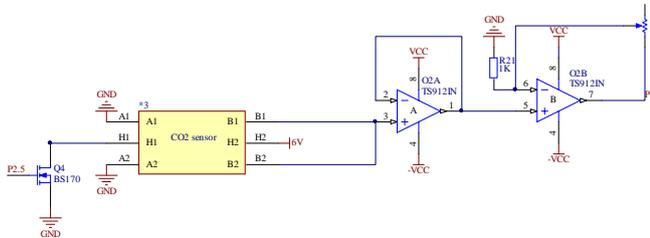
Figure 9: CO<sub>2</sub> sensor circuit schematic
