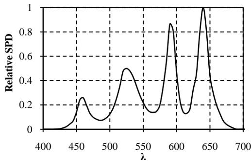
Figure 6: Relative SPD of the 4-band LED mixture (blue  $\lambda_b = 460$  nm, green  $\lambda_g = 530$  nm, amber  $\lambda_a = 590$  nm and red  $\lambda_r = 630$  nm),  $R_a = 95$ ,  $R_b = 86$ ,  $\eta_{\text{rad}} = 339$  lm/W, CCT = 3268K,  $R_{12} = 76$  (the blue sample).
