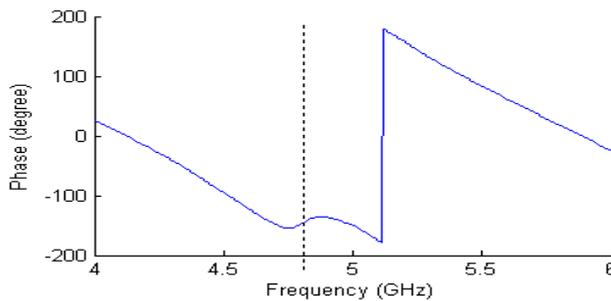
Figure 10. Measured phase variations. Resonance frequency 4.84GHz is shown by vertical line.
