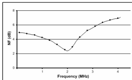
Fig. 11. Noise Figure variation with frequency.
