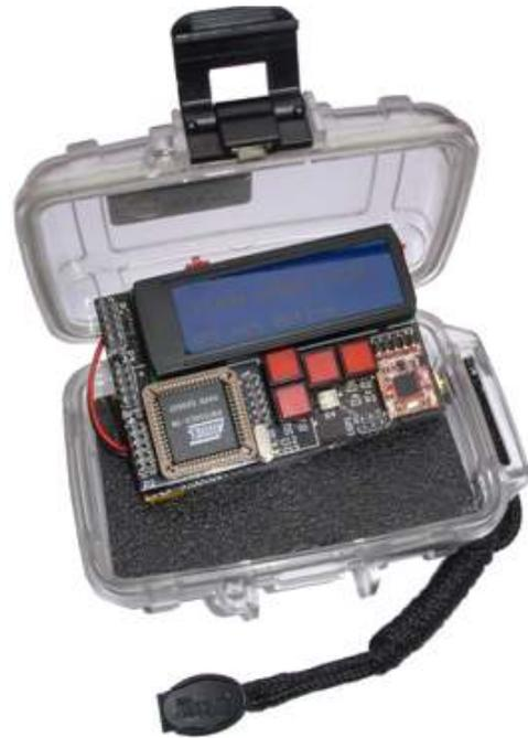
Figure 3 - The completed device inside the water proof case (Otterbox)
