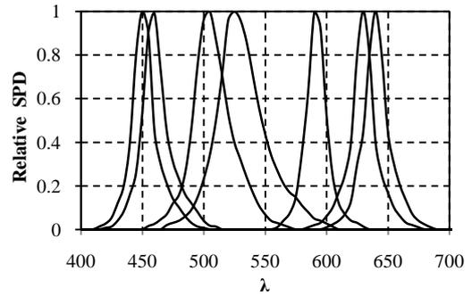
Figure 4: The spectral power distributions of the seven LEDs used in our experiments. [10]
