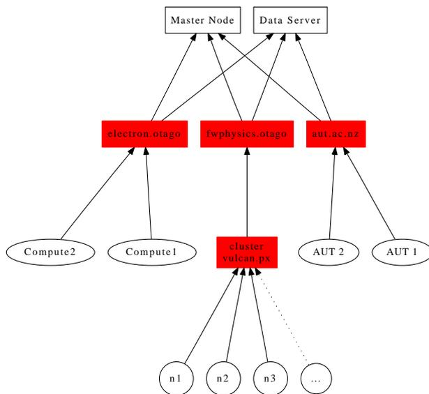
Figure 3: OGRE grid hierarchy showing firewalls, clients and clusters.
