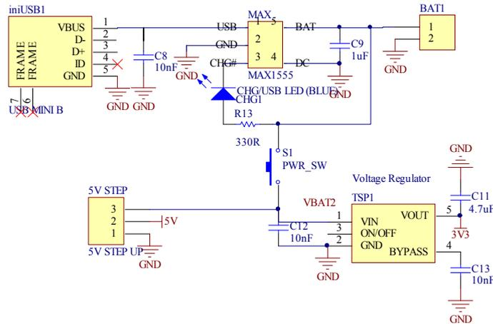
Figure 1- Battery charging (3.7V) circuit via USB (5V) and MAX1555, and regulated supply voltages.
