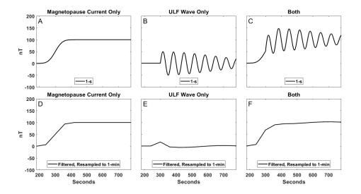
**Figure 8.** A) An example low latitude magnetic response to a solar wind pressure pulserelated magnetopause current intensification sampled at 1.0 Hz (solid black line). B) An example ULF wave generated by a pressure pulse sampled at 1.0 Hz. C) A superposition of the signals seen in A and B. D-F) The same signals as A-C, but after the application of a 60 s boxcar average.
