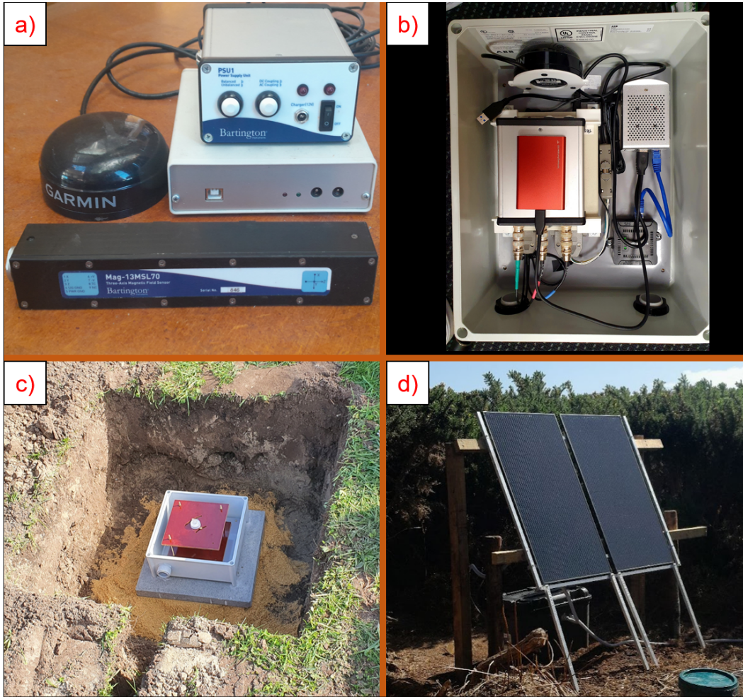
Figure 3. (a) Equipment used at the sites, including the Mag-13 at the front, the GPS unit on the left and the PSU atop the ADC on the right. (b) An example of the data logger box. The RPi was stored in a protective metal box (top-right), while a POE splitter brings power and ethernet to the setup. (c) A magnetometer chamber atop a concrete slab with the Tufnol baseplate inside pre-burial. (d) The solar panel setup of the Awarua magnetometer, with a larger data logger box below the panels. In this case, the solar panels were oriented to 60°N to ensure optimal solar charging in the winter months.
