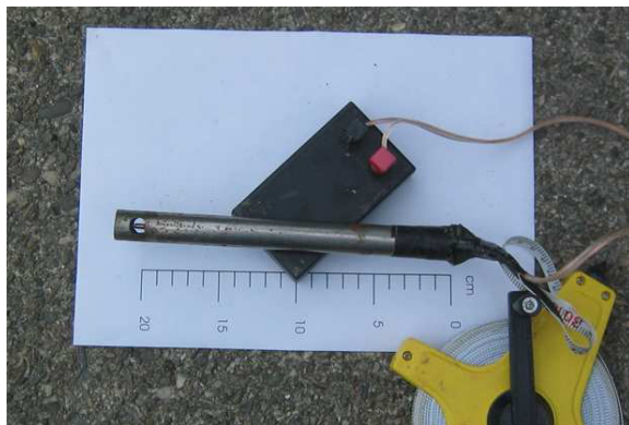
Figure 5: The sensor head connected to a tape measure and wiring, sitting on the box that houses the electronics.
