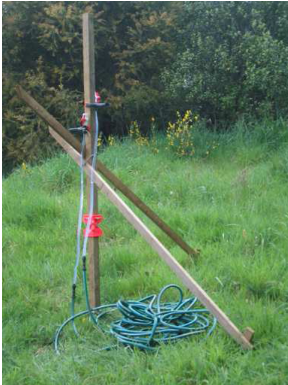
Figure 2: The hose level made up of a water-filled garden hose with clear tube ends, with both ends clamped to a post. A red post-level is visible, while foam on top of the water is just visible.
